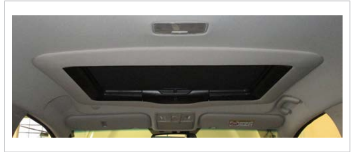
Fig. 04: Properly adjusted trim-shell carrier
