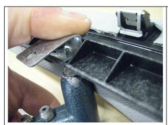
Attach bracket in position with pop rivets.
