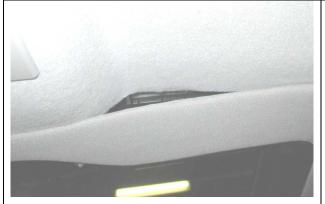
Substantial height difference in front, next to lowering in headlining, can result in a large gap when using the trimshell.
