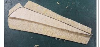
2. Cut away –without damaging fabric!- foam material along marking.
