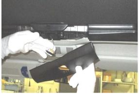
Turn switch to go through opening in switch cover.
