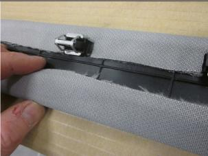
Peel off fabric at outer side (=without clips) only.
