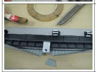
Prepare fabric around bracket for placing it back.
