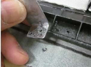
Remove drilling chips completely.
