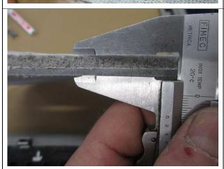
Measure thickness original headlining material at each determined bracket position.
