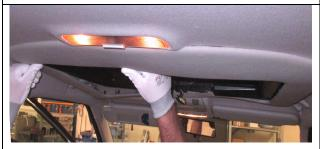
Push the clamps in the designated apertures in trimmingframe. Start at the rear...
